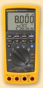
The Fluke-789 doubles your power giving you a multimeter and a loop calibrator in one tool.
